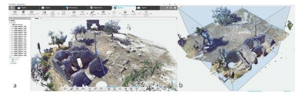
Fig.5 The program interface and the point cloud of the bath (a) and clipbox command (b)
