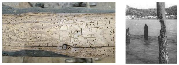
*Figure 1.* (a) Flight holes created by insects at the wooden beam; (b) Port Moresby, Papua New Guinea: CCA-treated hoop pine pilings destroyed by infestation in the intertidal zone by Sphaeroma triste [11].
