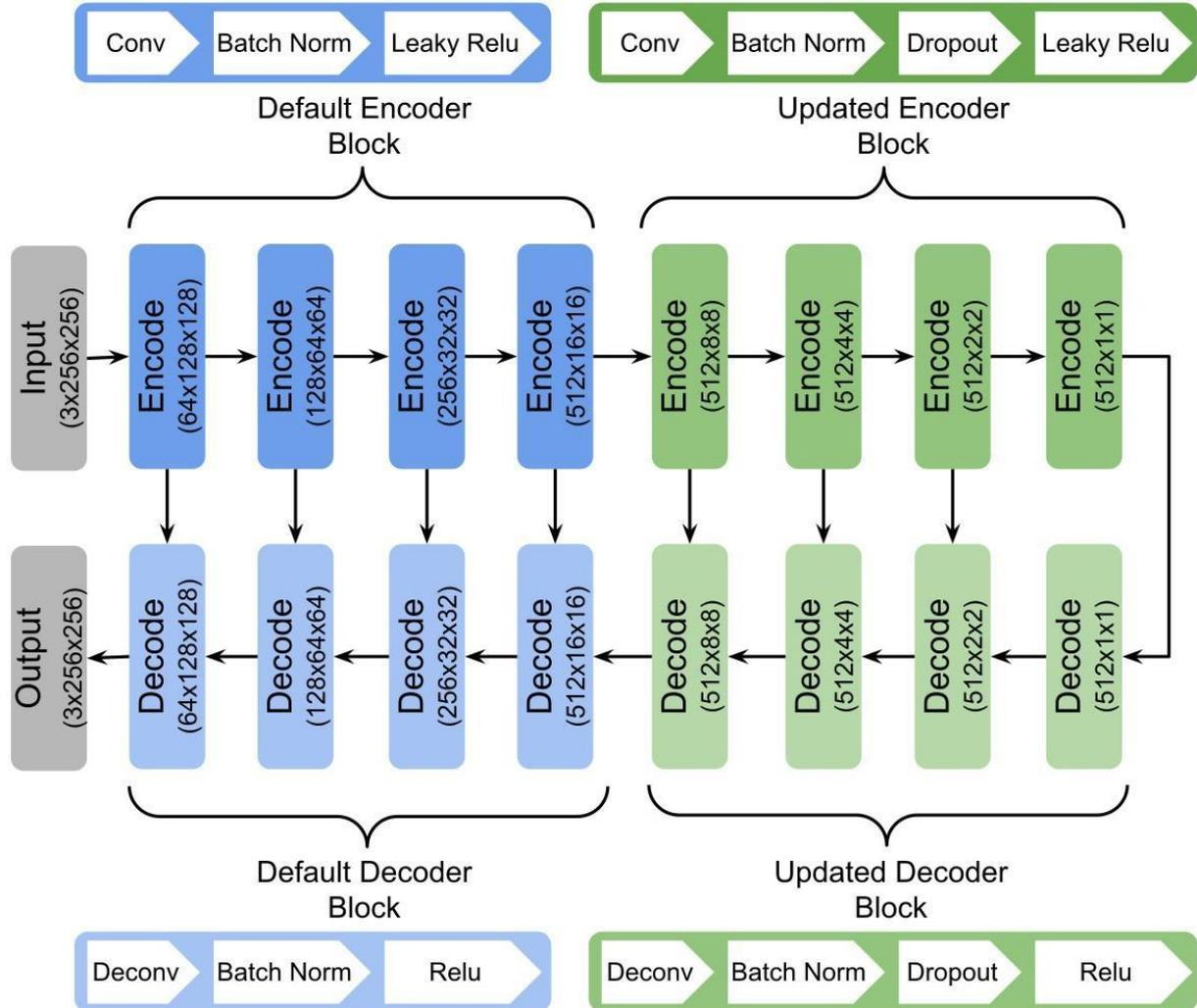
**Figure 5.** Updated version of Pix2Pix generator network architecture
