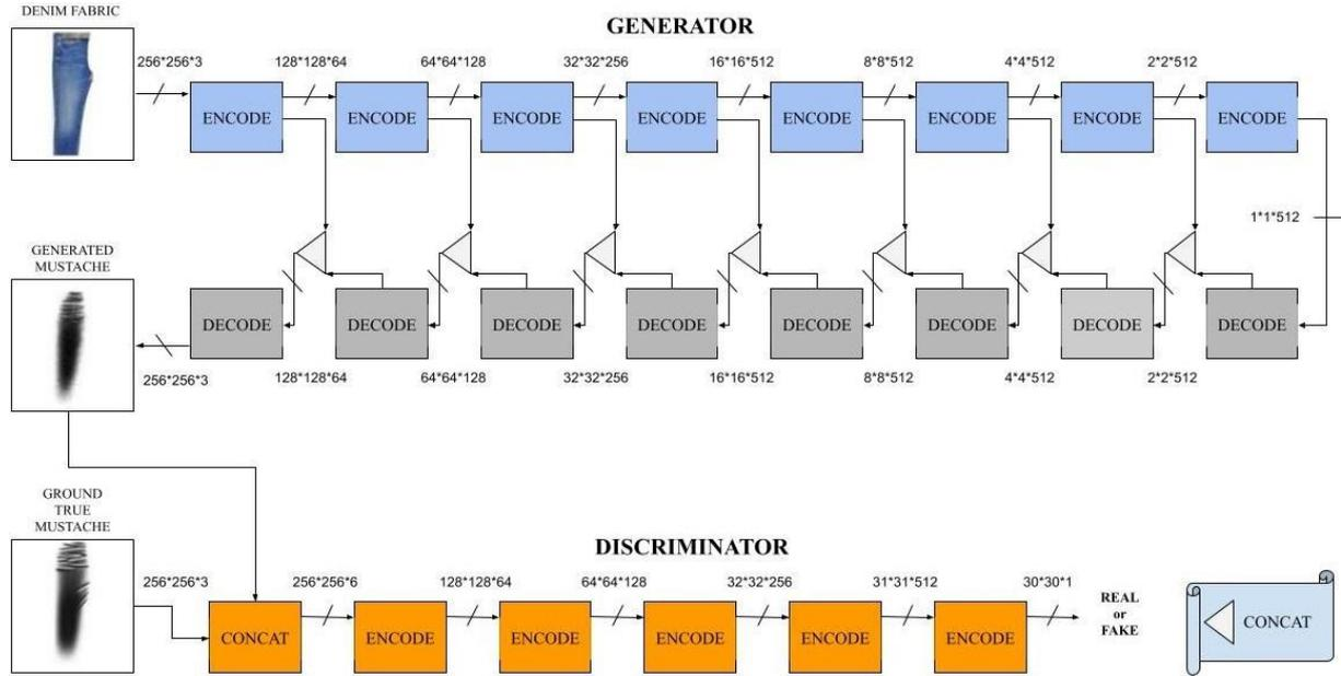
**Figure 4.** The use of Pix2Pix architecture in mustache pattern extraction
