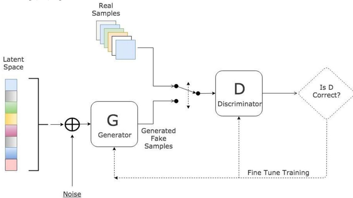
**Figure 2.** General schema of GAN architecture [14]
