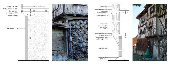
Figure 8. (a) Ground floor system detail of house number 23 (b) System detail of the first and second floors of the house number 63
