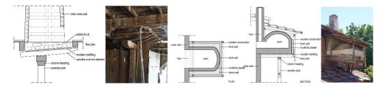
*Figure 17.* Oven detail of house number 71 B *Figure 18.* Oven plan and section detail of house number 34
