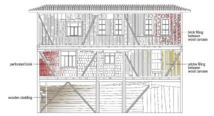
Figure 9. Facade drawing of house number 56 and display of different filling materials
