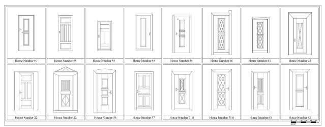
Figure 19. Types of room doors detected in the study area
