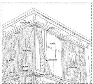
Figure 5. Perspective drawing of the wooden frame system of the house numbered 71B
