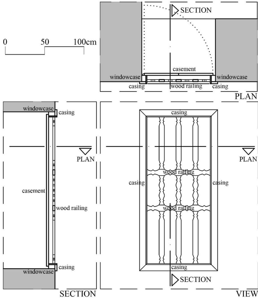
Figure 10. Wood railing window detail example
