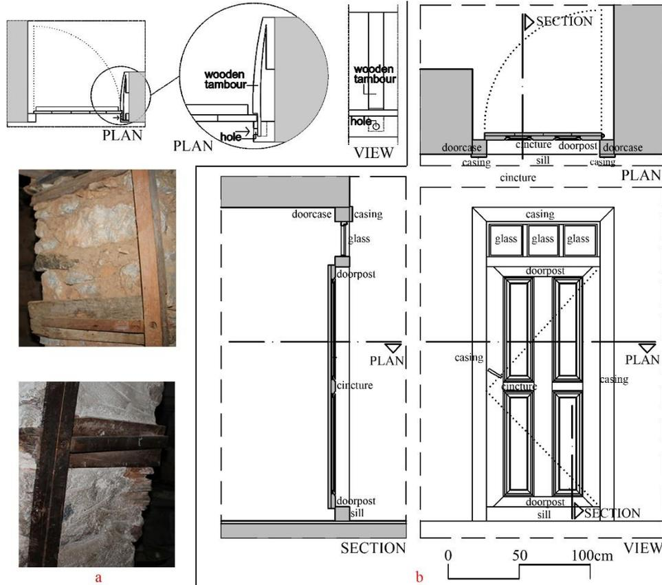
**Figure 9.** Door lock (a) and sample door details of traditional houses in Alanya's rural region
