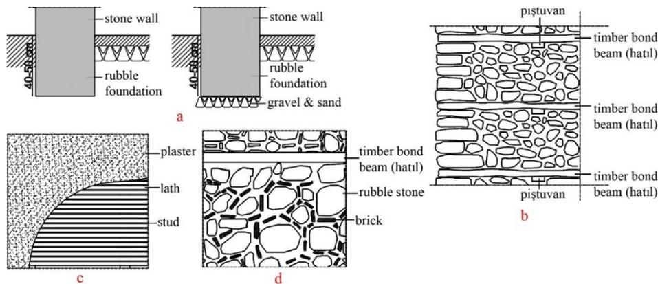
**Figure 1.** System details of traditional houses in Alanya's rural region ((foundation (a), drywall (b), timber-work (c) and nailing (d))
