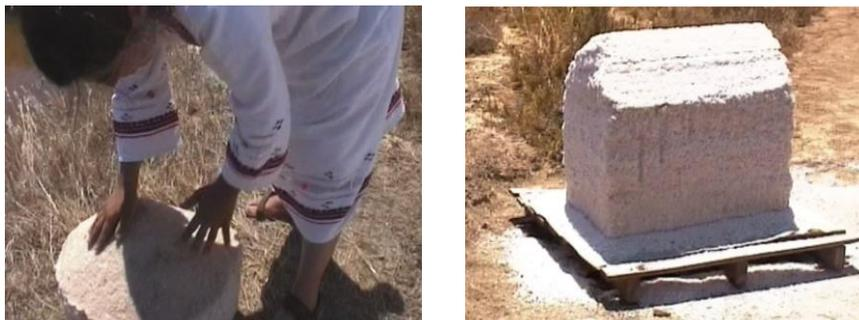
Fig. 2-3: Salt objects resulting from basket mould and wood formwork (Reaes Pinto, 2013).
