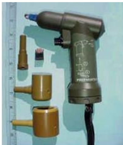
Figure 10: S4PE Surface Sampler Probe.
